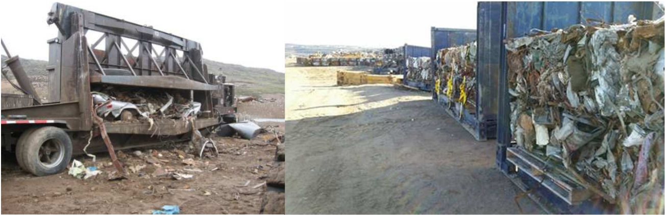
Photo 3: Vehicle crusher; container filled with scrap metal and end-of-life vehicles
