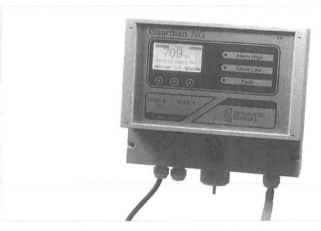
The NEW Guardian range of infrared gas monitors supplied by Edinburgh Sensors offers near-analyser quality, continuous sampling, measurement and display of target gas concentrations. The 'Guardian NG' range provides high accuracy detection and measurement of either  $CO_2$  or  $CH_4$  gases, where detection level ranges of between 0-3000ppm and 0-100% by volume are required.
